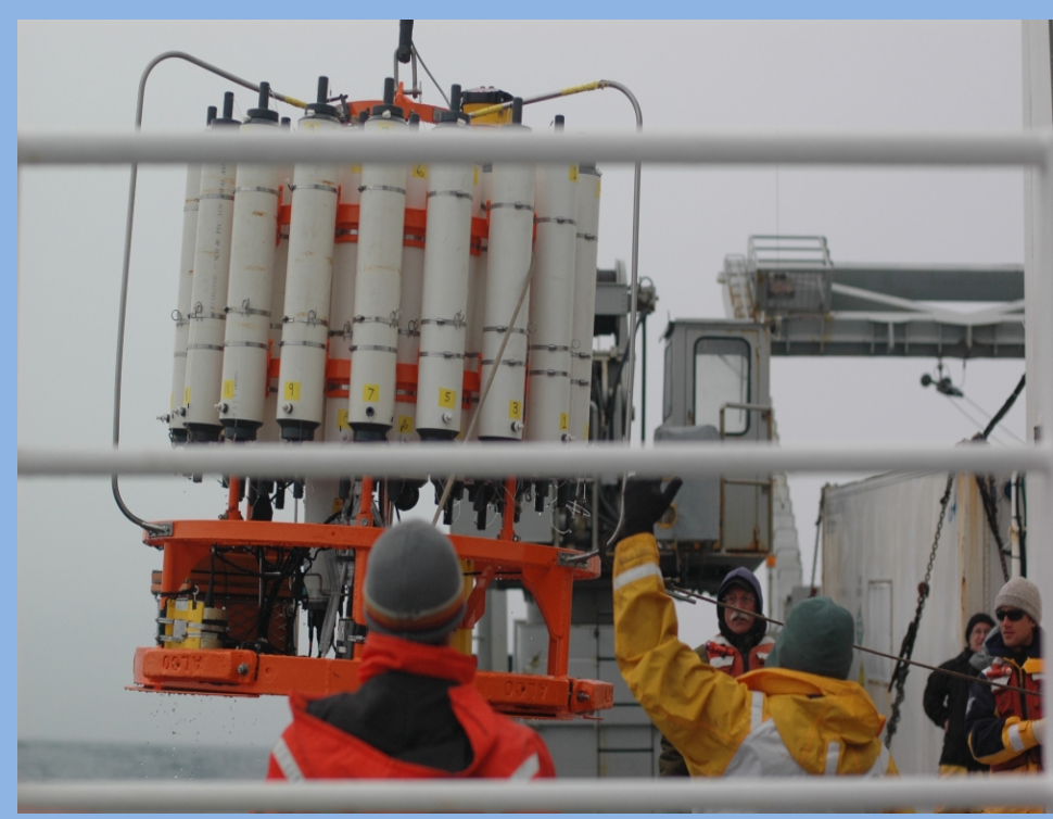
Figure 2. Today we see large CTD/rosette systems that add to the flushing problem, because of short soak times and because they entrain water as they are raised through the water column (courtesy of AWI).
